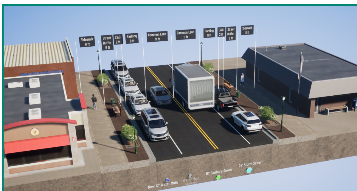
Figure 1: A 3-D rendering of a roadway can allow city planners to determine the best use of the right of way. Options like landscaping, street parking, bike lanes, and more can quickly be analyzed.
