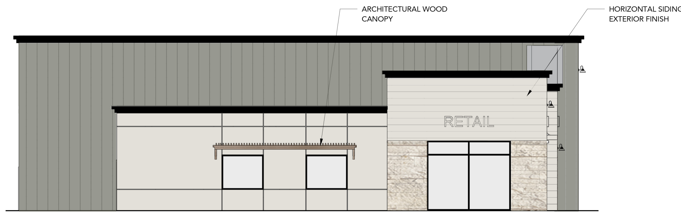
2 SOUTH ELEVATION - SOUTH RETAIL 1/8" = 1'-0"
